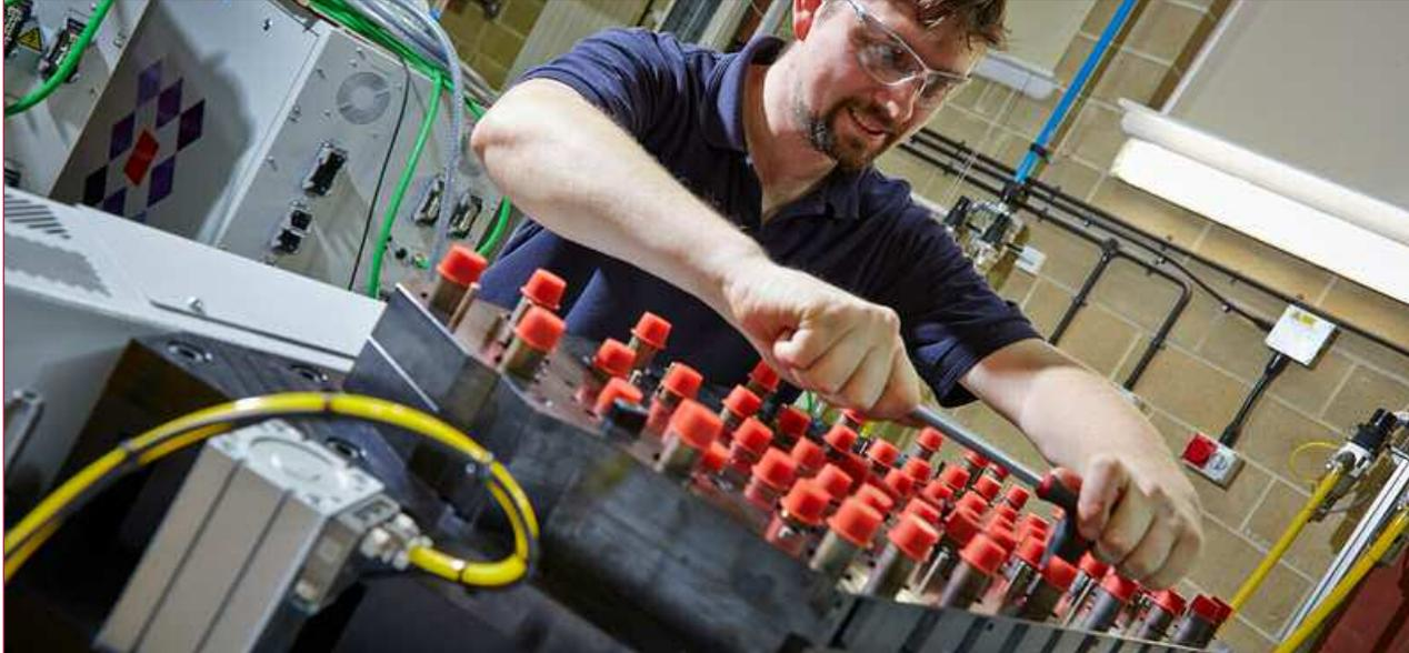
Compression mould tool build.
